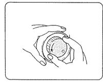
Release clutch by turning the clutch knob inside the hand wheel toward you.
